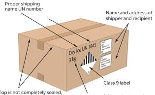
Top is not completely sealed, allowing gases to vent
