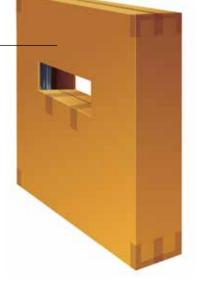
This design combines the use of a scored pad, a die-cut corrugated insert, and a moulded insert to help provide cushioning and bracing of the door inside the outer shipping container.
