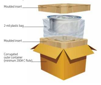
This design protects the rim from dents, scratches and abrasions. The moulded inserts are designed to fit multiple sizes.
