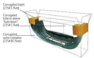
This design protects the fascia from scratches and abrasions. Additional poly-bag surface protection is optional.
