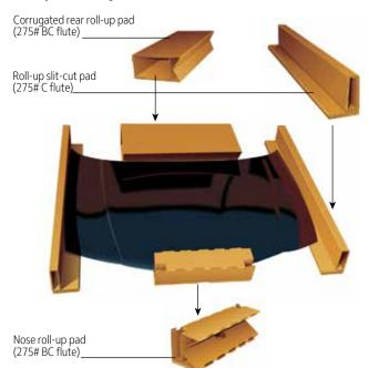
With this design, you centre the nose and rear roll-up pads and staple them to the inner flaps of the end-loaded full-overlap shipping container. Place the hood in the container followed by roll-up slit-cut pads. Close and tape.
