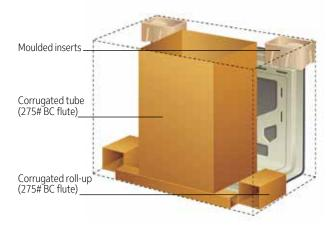
This design helps protect the trunk pack from external forces. Moulded inserts are used to create air cells and brace the trunk lid.
