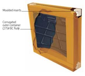
This design uses moulded pulp inserts on all four class A sides of the inner container to help provide cushioning.
