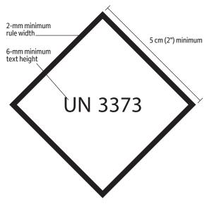
"Biological Substance, Category B" must appear in 6-mm-high text on the outer package adjacent to a diamond-shaped mark like the one shown here. The UN 3373 marking must be in the form of a square set at an angle of 45 degrees. Each side of the UN 3373 diamond should measure a minimum of 5 cm (2"). The width of the diamond rule line must be a minimum of 2 mm, and the letters and numbers must be at least 6 mm high.
